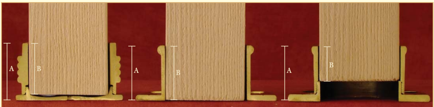
880 Concealed Recess Socket in Cross Section, showing how the pole fits into the socket
