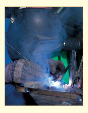
With in house welding and brazing facilities, Brass and Iron products, like brackets, swing arms and embraces can be fabricated to your specific requirements. Here we see a brass double pole bracket being brazed by our skilled technician.
